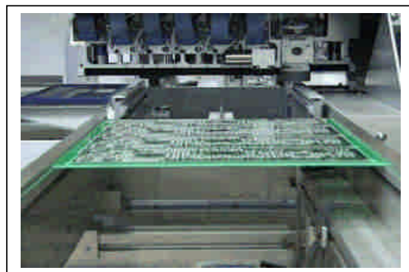
Fig 3 Head w 5 nozzles and camera
